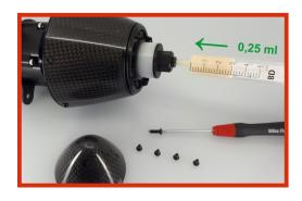
3. Press **0.25 ml** of the supplied lubricant into the hole in the shaft. We strongly recommend that you do NOT use different lubricant, only the lubricant supplied with the drive can be used.
