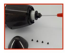
2. Unscrew a bolt from the gearbox shaft (lubrication hole).
