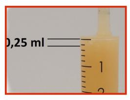
Marked volume **0.25 ml** intended for one lubrication interval. Do not exceed the recommended volume.
